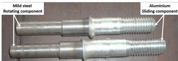
Fig. 2. Friction stud welded Al–MS specimen.
