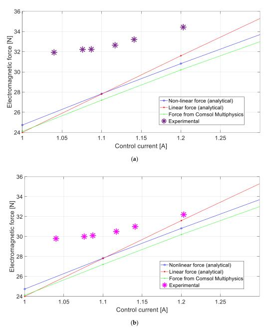
**Figure 23.** The resultant electromagnetic forces generated by the magnetic bearing for different values of the control current for the constant rotor–shaft raceway displacement equal to -0.06 mm with experimental results: coefficients  $k_x$  and  $k_i$  obtained analytically (**a**); coefficients  $k_x$  and  $k_i$  determined with the use of Comsol Multiphysics software (**b**).
