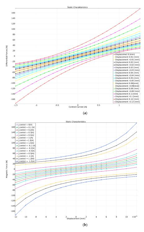
**Figure 14.** The static characteristics for different displacements of the rotorshaft raceway in the air gap (a) and various control currents (b).
