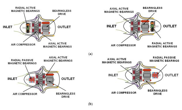
**Figure 1.** Concepts of the electric jet engine: configurations of jet engines with radial and axial active magnetic bearings and with a bearingless drive (a); configurations of a jet engine with one passive radial magnetic bearing, one axial active magnetic bearing and with a bearingless drive (b).
