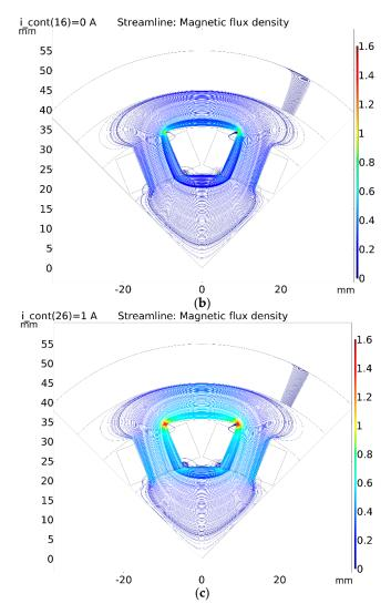
**Figure 8.** Streamline magnetic flux density for the control current of -1 A (**a**), 0 A (**b**), and 1 A (**c**).
