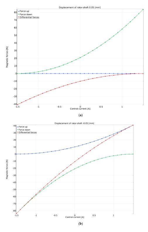
**Figure 13.** Magnetic forces vs. displacements of the rotor–shaft raceway equal to 0.05 mm (a) and -0.05 mm (b).
