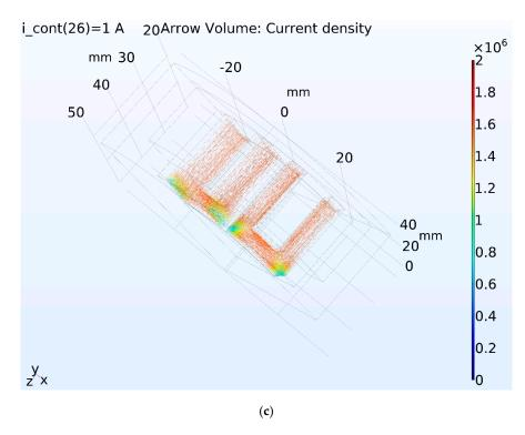
**Figure 7.** Current density for the control current -1 A (a), 0 A (b), and 1 A (c).
