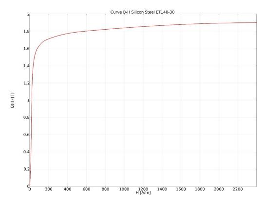
Figure 5. The magnetisation curve of silicon steel Et140-30.
