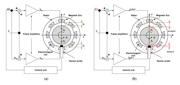
**Figure 2.** Active magnetic suspension: rotor in the operation point (a), rotor outside of the operation point (b).
