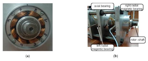
Figure 17. Laboratory object: (a) radial active magnetic bearing; (b) rotor–shaft support system.
