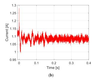
**Figure 18.** Time histories of the registered quantities: the rotor–shaft raceway displacement (a); the control current (b).
