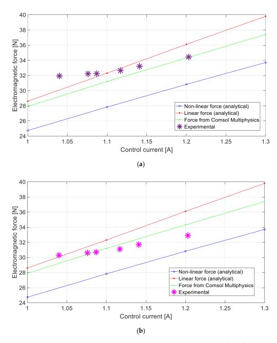
**Figure 22.** The resultant electromagnetic forces generated by the magnetic bearing for different values of the control current for the constant rotor–shaft raceway displacement equal to -0.04 mm with experimental results: coefficients  $k_x$  and  $k_i$  obtained analytically (a); coefficients  $k_x$  and  $k_i$  determined with the use of Comsol Multiphysics software (b).
