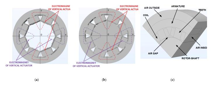
Figure 4. Electromagnetic actuators of the radial electromagnetic bearing—the armature of the actuator (a) and the rotor as an element of the actuator (b); reduced model of the radial electromagnetic bearing (c).
