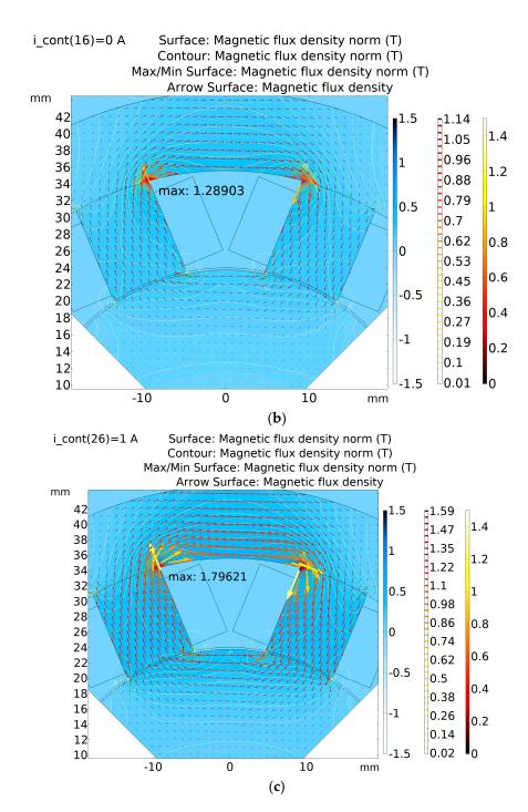
**Figure 9.** Magnetic flux density for the control current of -1 A (a), 0 A (b), and 1 A (c).
