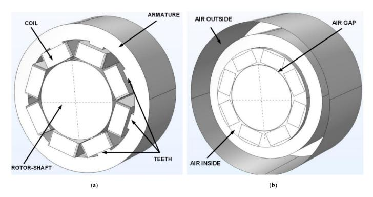
**Figure 3.** The geometrical shapes of the radial magnetic bearing components—magnetic circuits (a) air zones in the model (b).
