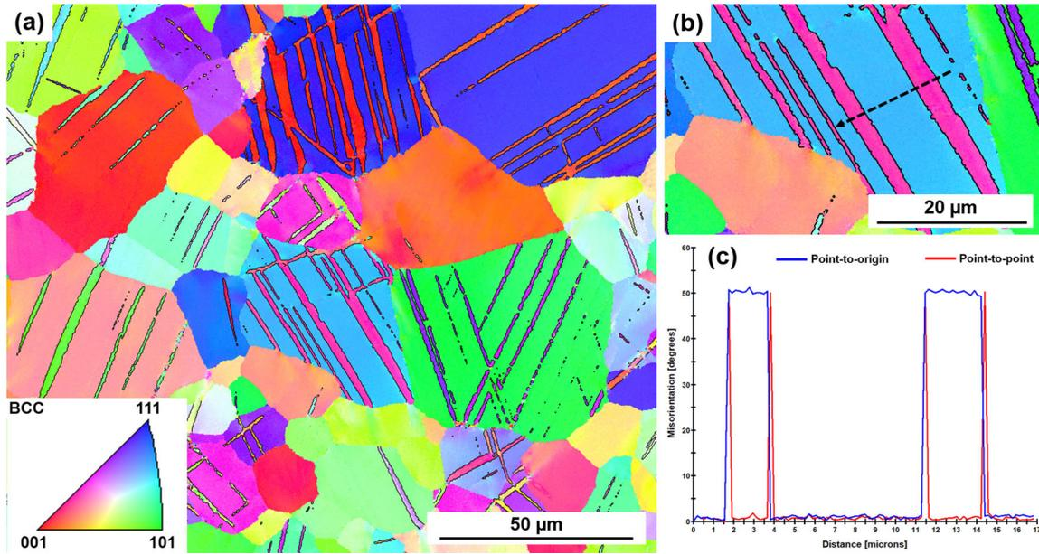
Fig. 10—EBSD orientation map of the deformed Ti-20Nb alloy (a), magnified area (b) with the corresponding misorientation profile (c). The  $\{332\}\langle 113 \rangle$  twin boundaries were marked by the black lines.
