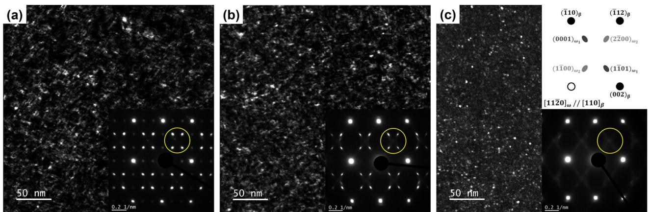
Fig. 3—The SAED patterns acquired along the  $[110]_{\beta}$  zone axis with the corresponding DF/TEM micrographs selecting the  $\omega$ -phase reflections (marked with the yellow circles) for Ti-14Nb (a), Ti-20Nb (b) and Ti-26Nb (c) alloys (Color figure online).
