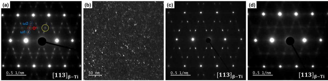
Fig. 4—The SAED patterns acquired along the  $[113]_{\beta}$  zone axis for Ti-14Nb (a), along with the corresponding DF image (b), Ti-20Nb (c) and Ti-26Nb (d). The presented DF image selecting the  $O'$ -phase reflection (marked with the yellow circle) (Color figure online).
