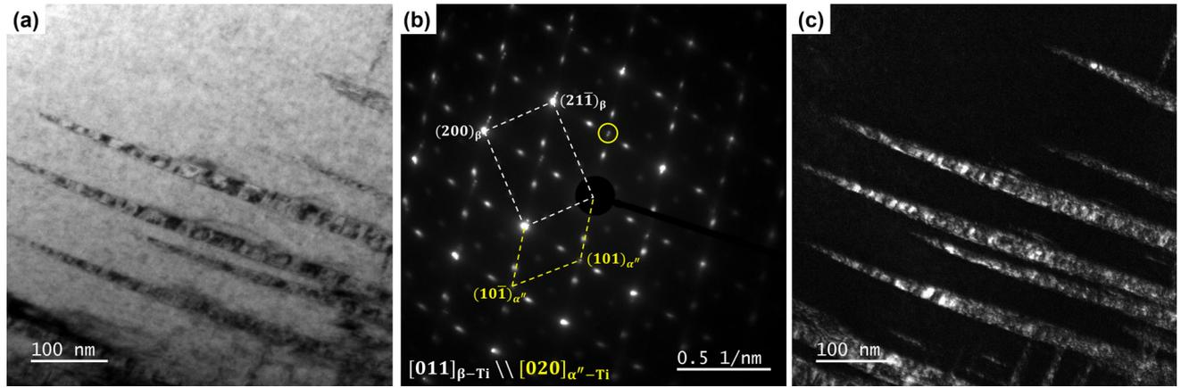
Fig. 2—BF/TEM micrograph of the Ti-14Nb sample (a) with the corresponding SAED pattern (b) and the DF/TEM image (c) selecting the  $\alpha''$ -martensite reflection, highlighted in the SAED with the yellow circle (Color figure online).
