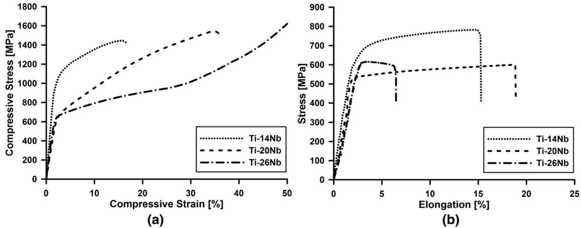
Fig. 5—Compression (a) and tension (b) stress–strain curves for the studied alloys.
