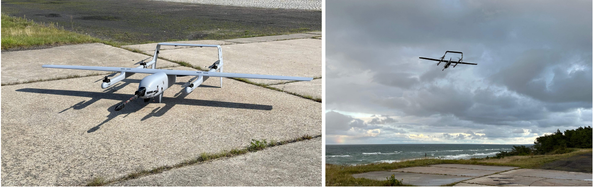
Figure 2: VTOL aircraft used for validation. The magnetometer system was installed on the nose.
