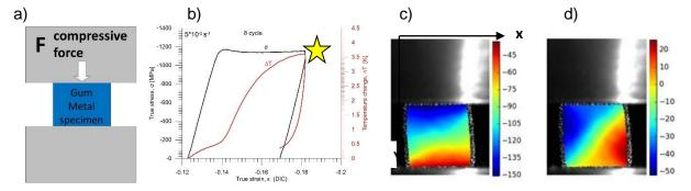
Compression of Gum Metal: a) scheme of the process, b) selected curve of stress  $\sigma$  and temperature change  $\Delta T$  vs. strain  $\varepsilon$  during the loading-unloading, DIC displacement fields in the end of loading: c) in loading direction, d) in direction perpendicular to Gum Metal loading.
